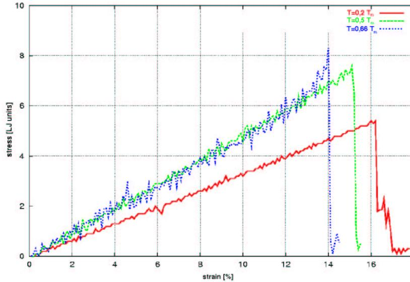
**Fig. 4.** Stress-strain curve for various temperatures.
