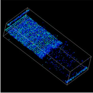
**Fig. 1.** Visualization of the dislocation line and the stacking fault. Only atoms with a large potential energy compared to the initial value are plotted.
