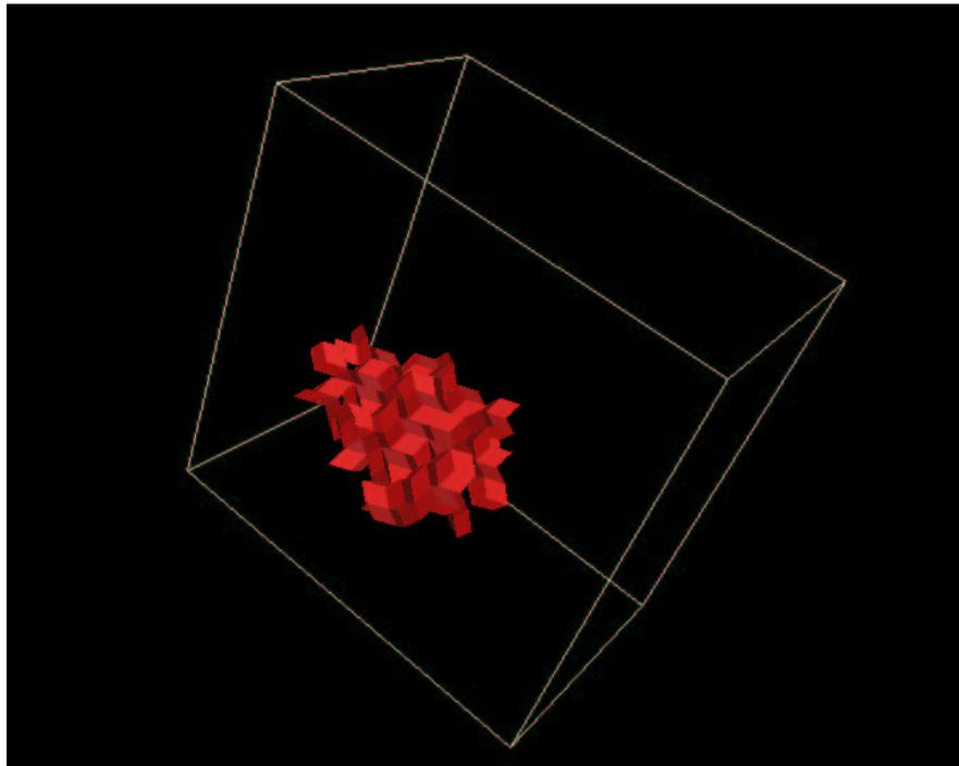
**Fig. 3.** Visualization of the boundary surface between defective and undefective regions. Rhombohedra with distorted bonds form the defective region.
